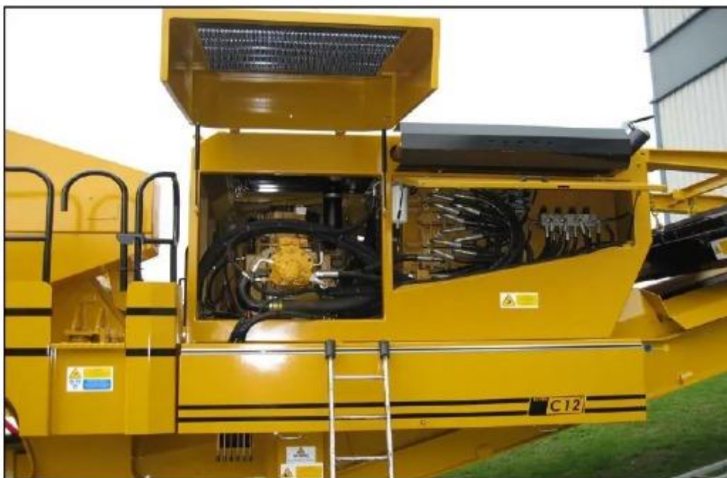
Caterpillar C-9 Powerpack- easy access for maintenance and service
