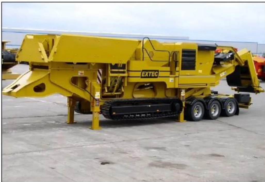
Optional bogie system - eliminates the need for low loader
