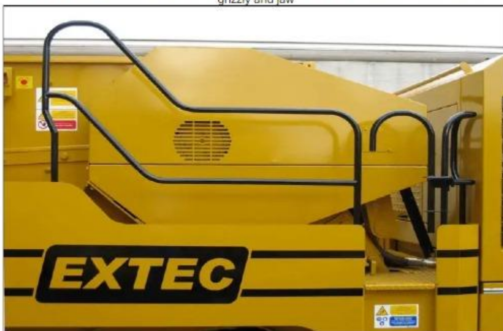
Maintenance platforms are provided on the right hand side of the crusher
