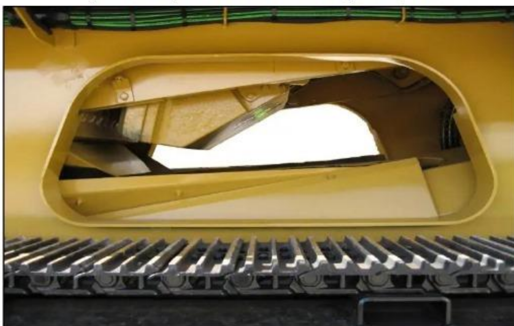
Large gap between discharge point of crusher and conveyor eliminates blockages and facilitates cleaning.
