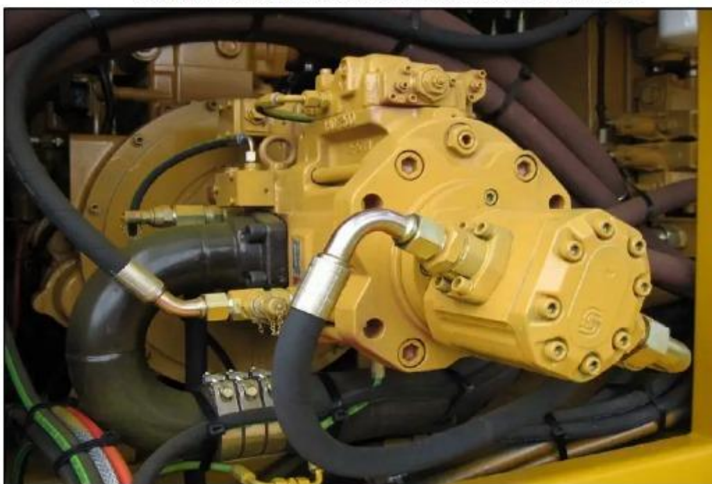
Caterpillar C-9 Powerpack- easy access for maintenance and service
