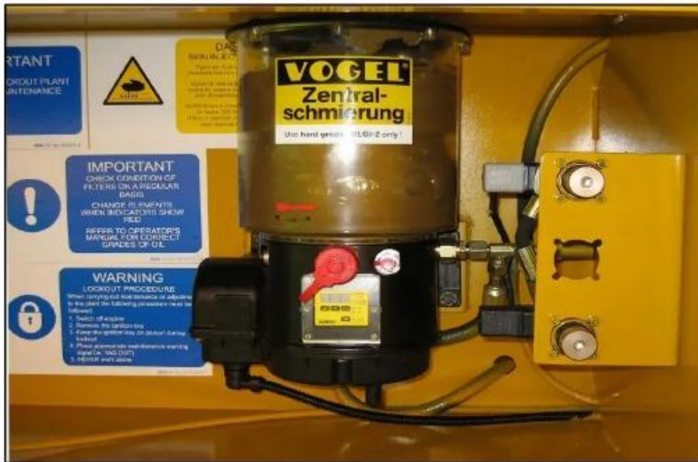
SKF automatic lubrication – reduced wear and downtime
