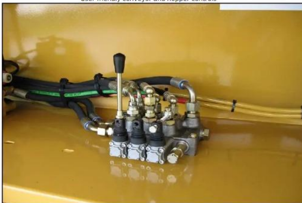
Extended main conveyor control
