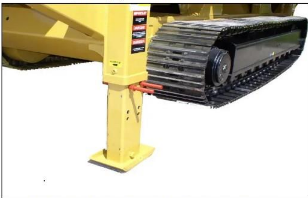
Machine raises on its hydraulic legs to facilitate cleaning and servicing of tracks
