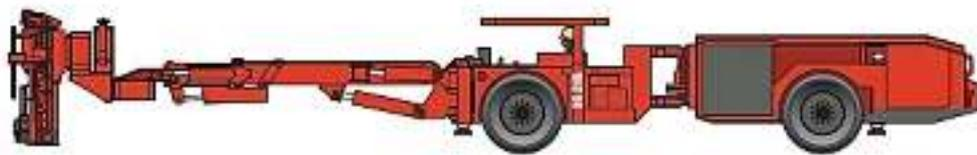
Sandvik DS210L-M is a fully mechanized one man operated electro hydraulic low profile bolting machine for rock reinforcement in excavations with headroom as low as 1.6 m.
