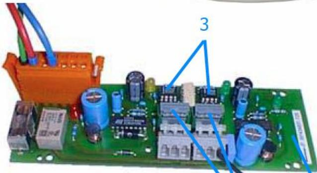
Platine for secondary power supply
